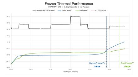
Frozen thermal perfomace of HydroFreeze compared to HydroFreeze alternatives. Test was executed with 3000 grams of coolants, no payload and the PHARMA4 EPA box. Full test results are available upon request.
